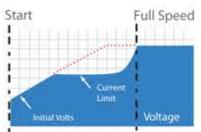
Voltage Ramp with Current Limit
