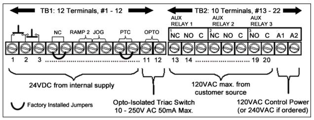
Figure 4.2: Control Terminal Blocks
