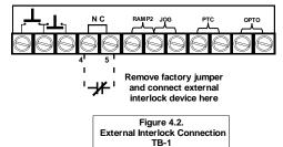
TB1 provides a connection point for an external dry (voltage free) N.C. (Normally Closed) interlock device between terminals 4 and 5. Examples where this interlock connection would be used include low oil, high temperature, or excess vibration dropout from user supplied devices. A factory-installed jumper is provided which allows the **VMX Series** unit to operate if external interlocks are not used. If this jumper is removed and an interlock is not used, the VMX Series unit will not function.
