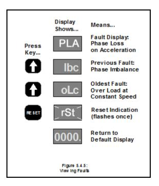
This Fault History can only be accessed during a fault condition. While the active fault number is being displayed, use the Up and Down Arrow keys to scroll through the Fault History. An additional Fault History complete with Time and Date stamps is also available for viewing at any time in **F085** through **F093**.
