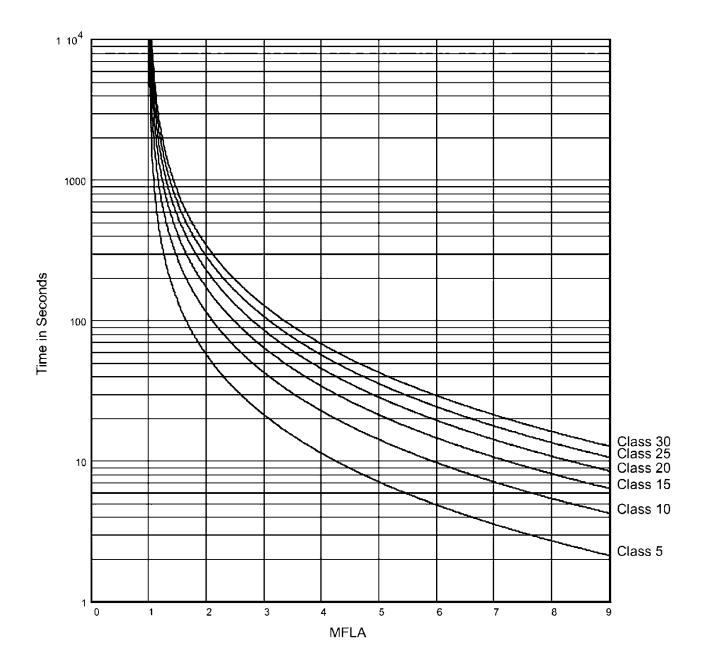
Note: Factory default setting is Class 10 for both Start and Run Overload Protection
