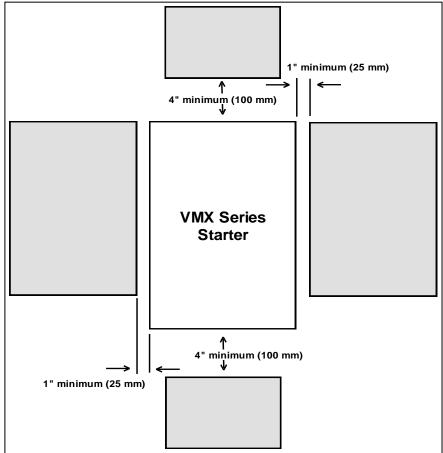
Figure 2.5: VMX minimum mounting clearances
