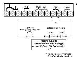
4.2.6.a External Over Load Relay Connection
