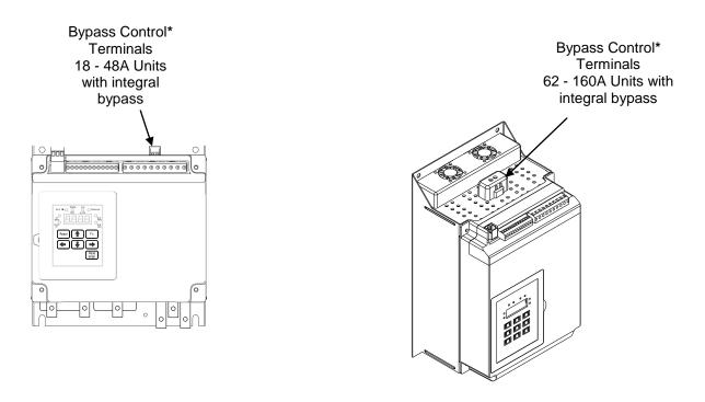
Note: Use these terminals only when separate control of the Bypass Contactor is necessary.
