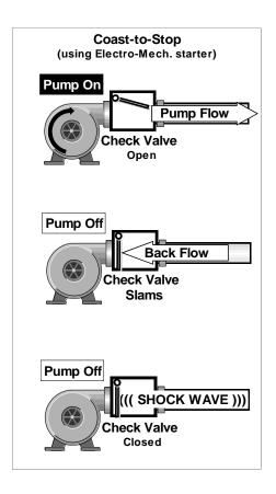
Pump-Flex® Deceleration (Soft Stop) is a unique feature of Motortronics Solid State Soft Starters. It provides a slow decrease in the output voltage, accomplishing a gentle decrease in motor torque during the stopping mode. This is the **OPPOSITE OF BRAKING** in that it will take **longer** to come to a stop than if the starter were just tuned off.
