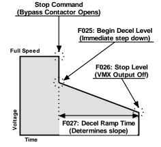
Figure 5.6.5: Pump-Flex Decel Ramp Settings
