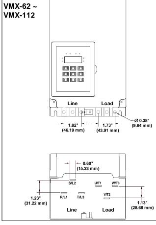
Figure 2.6.1 Critical clearances for bus tab connections
