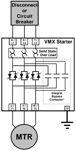
Figure 4.1: VMX Power Connections
