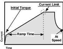
Figure APP 1.3: Current / Torque Ramp
