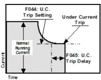
current of any phase drops below **F044** for more than 2 seconds, the starter will trip.
