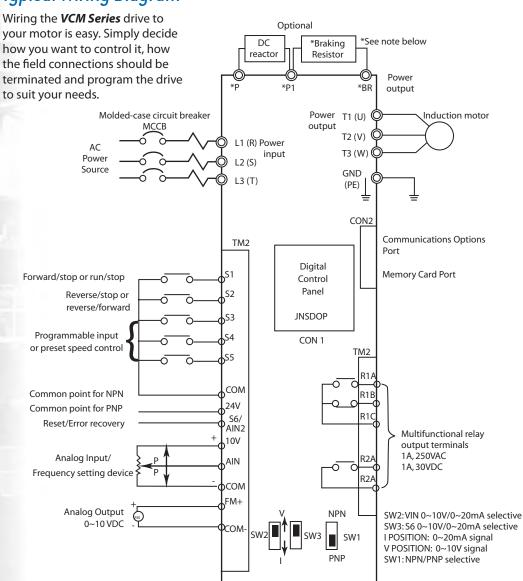
Diagram applies to models rated up to 10HP at 240V and 15HP at 480V. Contact factory for power schematic for larger sizes.
