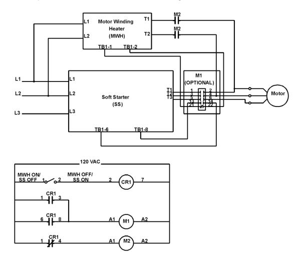
Wiring Diagram for units rated at 25 Amps
