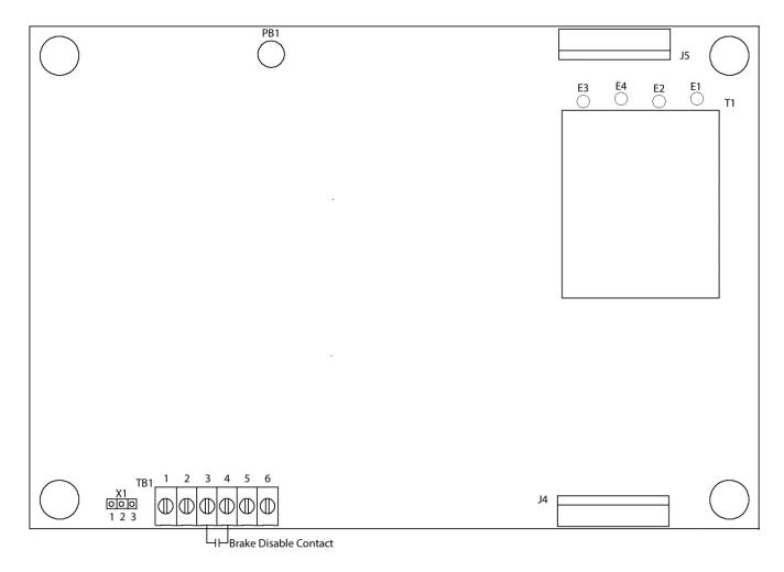
**NOTE:** The Brake Disable can and should be used to disable the ABC Series brake in the event of a motor thermal overload by wiring a normally open contact from the overload relay to these terminals. This will prevent the brake from operating if a motor overload trip condition occurs.
