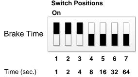
**NOTE:** Stop times shorter than 4 seconds will not allow enough time for the Zero Speed Sensing circuit to accurately sense that the motor has stopped. The Brake Time settings must be used in applications that require brake times less than 4 seconds.
