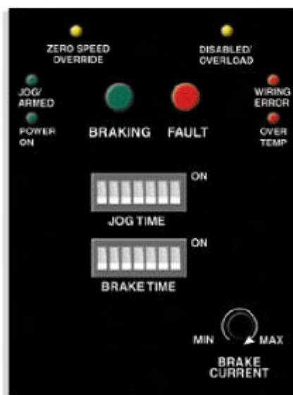
Operator Interface Module
